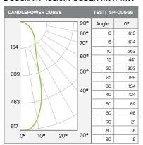
Delivered Lumens: 553 Luminaire Watts: 13 LER: 43 CP @ 0° (Nadir): 613 Beam Angle: 38.2° CRI: 83
