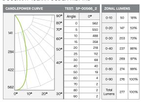
Delivered Lumens: 277 Luminaire Watts: 13 LER: 21 CP @ 0° (Nadir): 562 Beam Angle: 34.9° CRI: 83 13L / OSD - 83 CRI
