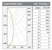
Delivered Lumens: 1881 Luminaire Watts: 23.7 LFR: 79
