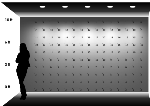
5 LUMINAIRES 3' away from wall 3' between luminaires
