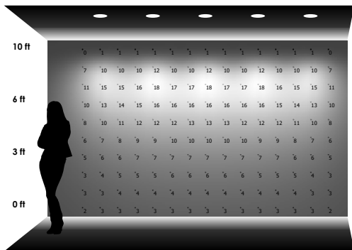
5 LUMINAIRES 3' away from wall 3' between luminaires
