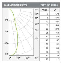
Delivered Lumens: 442 Luminaire Watts: 13 LER: 34 CP @ 0° (Nadir): 578 Beam Angle: 37.8° CRI: 83
