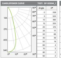
Delivered Lumens: 280 Luminaire Watts: 13 LER: 22 CP @ 0° (Nadir): 538 Beam Angle: 35.4° CRI: 83
