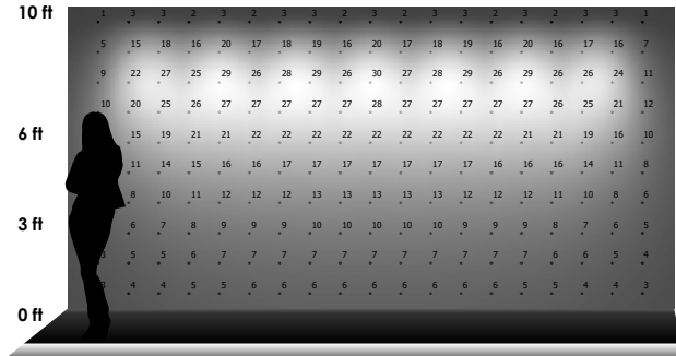
7 LUMINAIRES 2' - 6" away from wall 2' - 6" between luminaires
