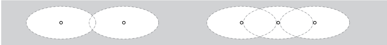
64° x 27° Beam Angles oriented for linear, overlapping light pattern
