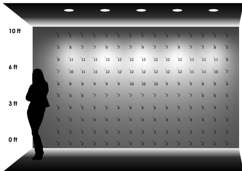
5 LUMINAIRES 3' away from wall 3' between luminaires
