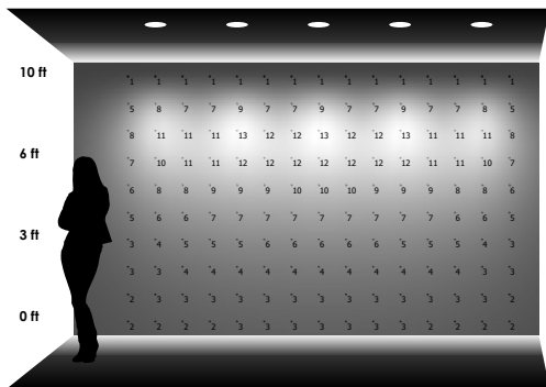
5 LUMINAIRES 3' away from wall 3' between luminaires
