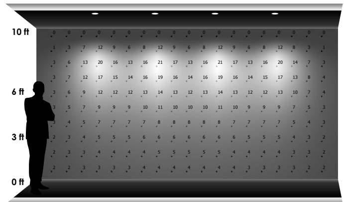
4 LUMINAIRES 3' away from wall 4' between luminaires
