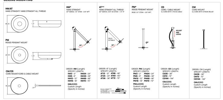
\*MAXIMUM ONE PIECE STEM LENGTH IS 72". \*\*MAXIMUM ONE PIECE STEM LENGTH IS 36", LONGER LENGTHS ARE POSSIBLE USING MULTIPLE STEMS AND COUPLERS. \*\*ORDER IN 12" INCREMENTS, ODD SIZES MAY BE FIELD CUT
