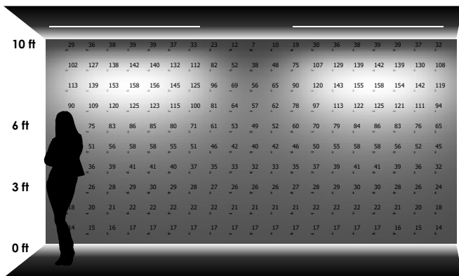
TWO LUMINAIRES 2'-0" away from wall 10'-0" on center
