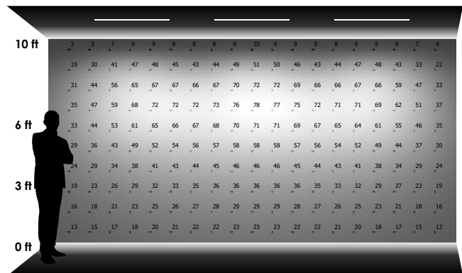
THREE LUMINAIRES 3'-0" away from wall 6'-0" on center
