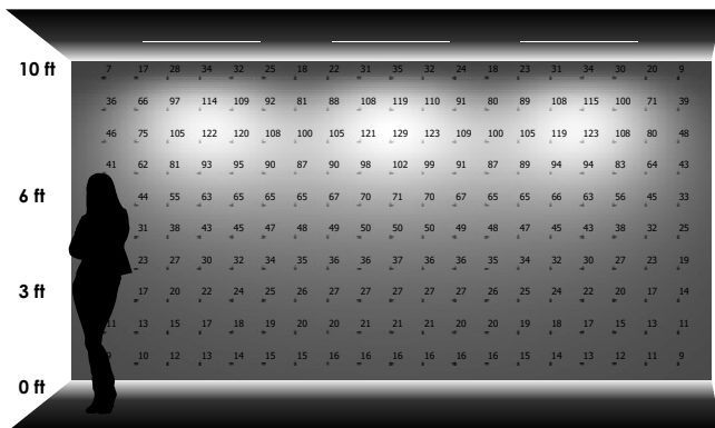
THREE LUMINAIRES 2'-0" away from wall 6'-0" on center
