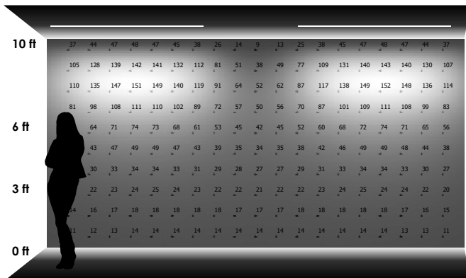
TWO LUMINAIRES 2'-0" away from wall 10'-0" on center
