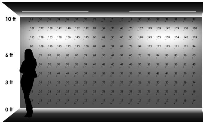
TWO LUMINAIRES 2'-0" away from wall 10'-0" on center
