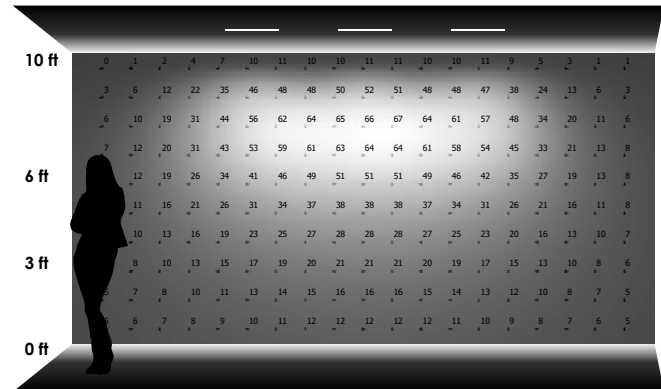
THREE LUMINAIRES 2'-6" away from wall 4'-0" on center
